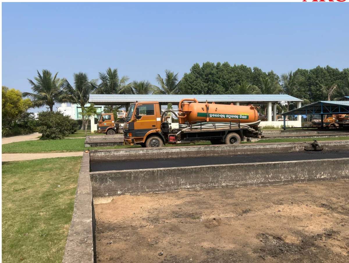
Figure 2: Desludging truck used by women sanitation workers at a faecal sludge treatment plant in Cuttack, India (Photo © Amita Bhakta)
